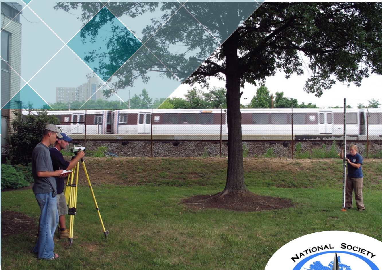
A Metro train whizzes past as Matt Whitehead, Dave Simms and Teresa Combs perform a peg test with a digital level.
